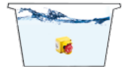
IP67: Submersion to one meter for 30 minutes.
